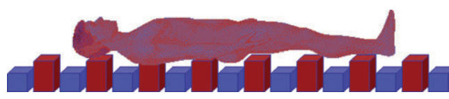
Figure 4 When movable parts move to their lowest position, fixed part could hold the entire patient's weight.
