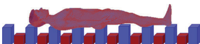
Figure 3 When movable parts move to their highest position, it could hold the entire patient's weight.
